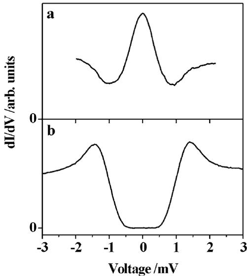
**Fig. 3.** **a** Differential conductance spectrum of superconducting NbSe<sub>2</sub> acquired after stabilising the feedback at 40 pA and +4 mV at a temperature of 210 mK. (This curve is an average of 128 individual curves.) **b** Differential conductance spectrum acquired in the centre of a vortex at 0.2 T and 110 mK after stabilising the feedback at 50 pA and +3.5 mV
