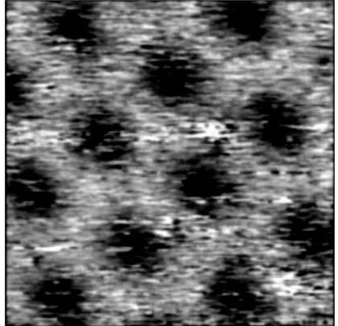
**Fig. 4.** 500  $\times$  500 nm image of the Abrikosov flux lattice formed with a 0.5 T field applied perpendicular to the sample
