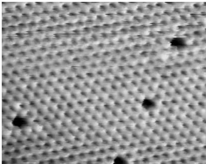
**Fig. 2.** Unfiltered  $7 \times 5.6$  nm atomically resolved constant-current image of  $\text{NbSe}_2$  acquired at 190 mK
