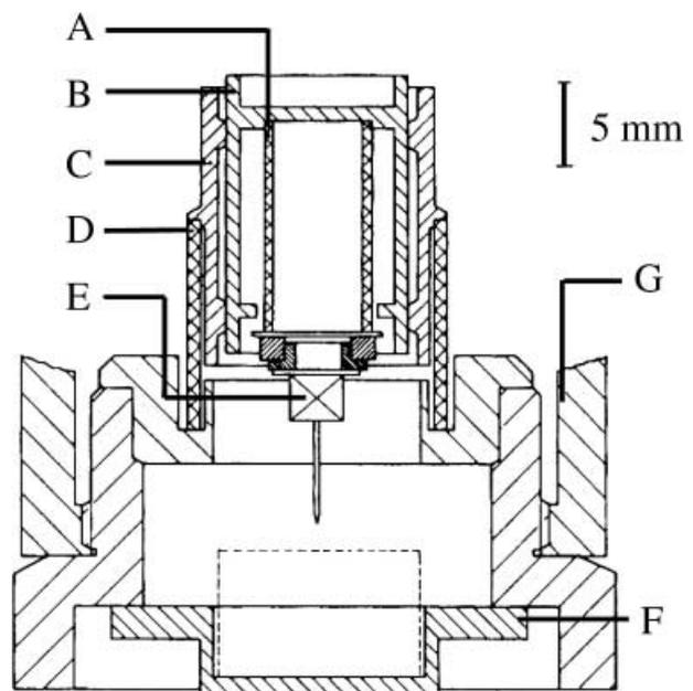
**Fig. 1.** Design of the STM head: (A) scan piezo-tube, (B) plunger, (C) leaf spring, (D) outer coarse-approach piezo, (E) tip holder, (F) sample holder, (G) STM body
