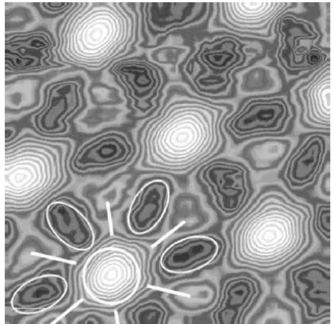
**Fig. 5.** Real-space image of the local density of states at 0 V of a 400  $\times$  400 nm area containing seven vortices, measured at 0.4 T and 125 mK
