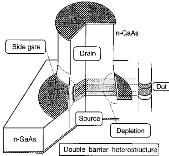
**Figure 9.1.** Schematic of the quantum dot in a vertical device.
