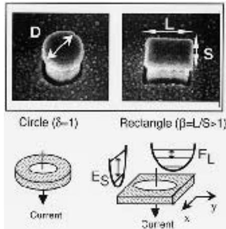
**Figure 9.2.** Scanning electron microscope (SEM) images showing submicrometre circular and rectangular mesas, and schematic diagrams of the resulting circular and elliptical shaped dots in the mesas.
