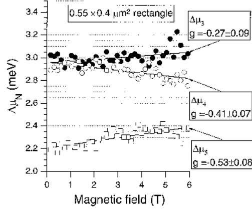
**Figure 9.9.** Zeeman shift of the levels,  $\mu(3)$ ,  $\mu(4)$  and  $\mu(5)$ , for the elliptical dot in the  $0.55 \times 0.4 \mu\text{m}$  rectangular mesa (X) [16]. The straight lines are fits to the data, which are used to estimate the electronic  $g$ -factor.
