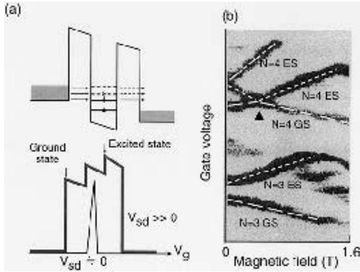
**Figure 9.6.** (a) Energy diagram and tunnelling current with a finite voltage is applied between the source and drain. (b) Derivative of the tunnelling current,  $dI/dV_g$ , as a function of gate voltage and magnetic field measured for the circular mesa (not W) with  $V_{sd} = 1.6$  mV. Changes in the grey scale indicate changes in the current amplitude. The white long-dashed curves indicate the GSs, the first and second ESs are shown by the white dotted-, and chain curves.
