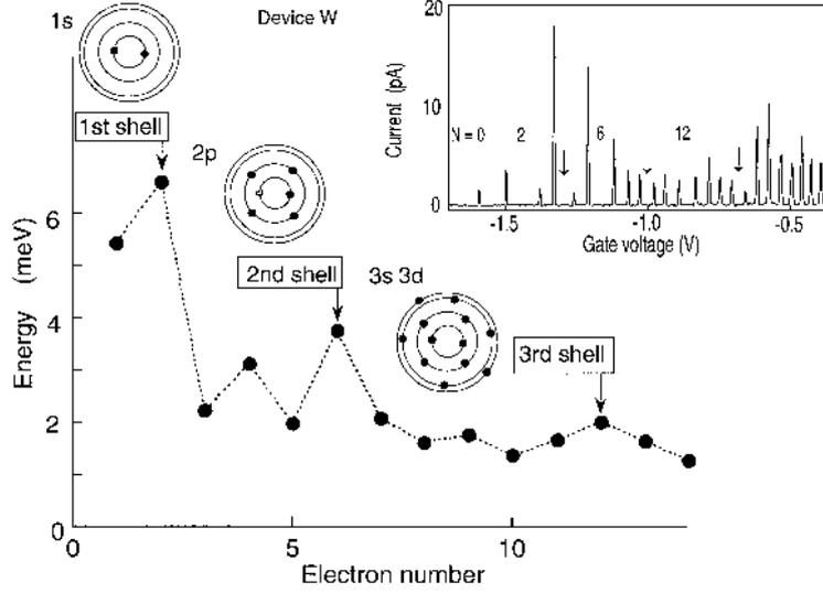
**Figure 9.3.** Change of the electrochemical potential,  $\mu(N+1) - \mu(N)$ , as a function of electron number,  $N$  [4]. Inset: Coulomb oscillations in current versus gate voltage at  $B = 0$  T measured at 50 mK.
