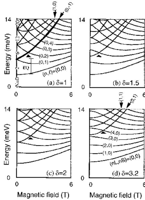
**Figure 9.4.** Calculated  $B$ -field dependence of the first ten single-particle energy levels for a circular dot with  $\delta = 1$ , and (a) for elliptical dots with  $\delta = 1.5, 2$  and  $3.2$ , (b)–(d) [5].
