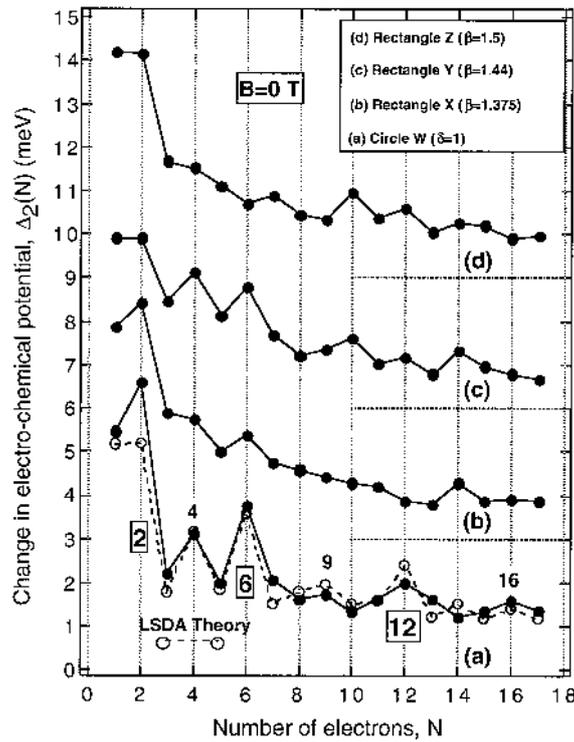
**Figure 9.7.**  $\Delta_2(N)$ , for the circular mesa W, (a) and the three rectangular mesas X, Y, and Z, (b)–(d) [7, 14]. The traces are offset vertically by 3 meV for clarity. The fit for W is given by a local spin-density approximation (LSDA) (see figure 9.10).
