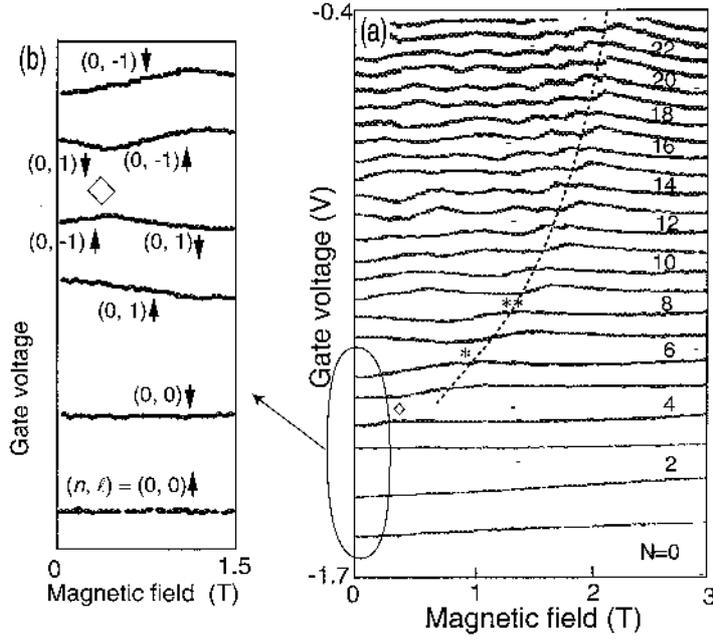
**Figure 9.5.** (a)  $B$ -field dependences of current peak positions measured for the device (W) whose Coulomb oscillations are shown in figure 9.3 [4]. (b) Magnified plot of the  $B$ -field dependences of the peak positions for the first six current peaks. The corresponding F–D states are indicated by  $(n, \ell)$  quantum numbers, and by  $\uparrow$  or  $\downarrow$ , where  $\uparrow$  or  $\downarrow$  is a state with an up-spin or a down-spin, respectively.
