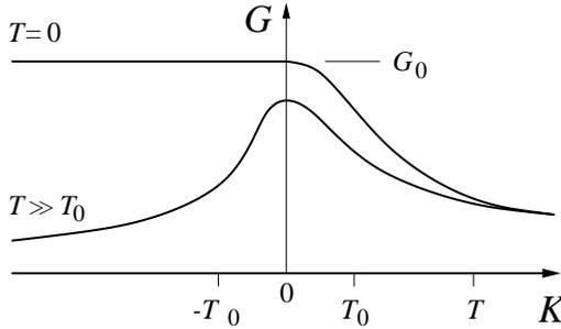
**Fig. 3.** Linear conductance near a singlet-triplet transition. At high temperature  $G$  exhibits a peak near the transition point. At low temperature  $G$  reaches the unitary limit at the triplet side of the transition, and decreases monotonously at the singlet side. The two asymptotes merge at  $K \gg T, T_0$ .
