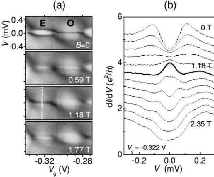
**Fig. 11.** (a) Evolution with magnetic field of adjacent even (E) and odd (O) features of the type seen in Fig. 10. (b)  $dI/dV$  vs  $V$  traces at the center of the E region, at  $V_g = -0.322$  V. The trace at  $B = B^* = 1.18$  T (bold line) corresponds to the dotted line in (a). The traces are offset from each other by  $0.4 e^2/h$  for clarity.
