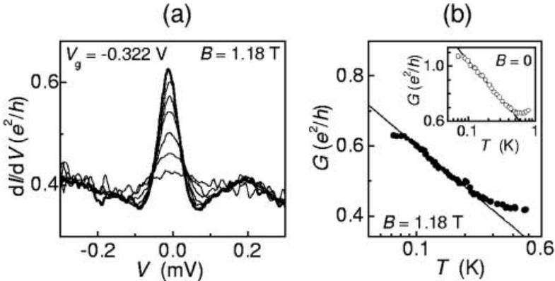
**Fig. 12.** (a) Temperature dependence at  $B = B^*$ . Here  $T$  = base (bold line), 100, 115, 130, 180, 230, and 350  $mK$ . (b) Temperature dependence of the linear conductance  $G$  ( $dI/dV$  at  $V = 0$ ) at  $B = B^* = 1.18 T$ . For comparison,  $G(T)$  in the center of one of the O-type ridges at  $B = 0$  is shown in the inset.
