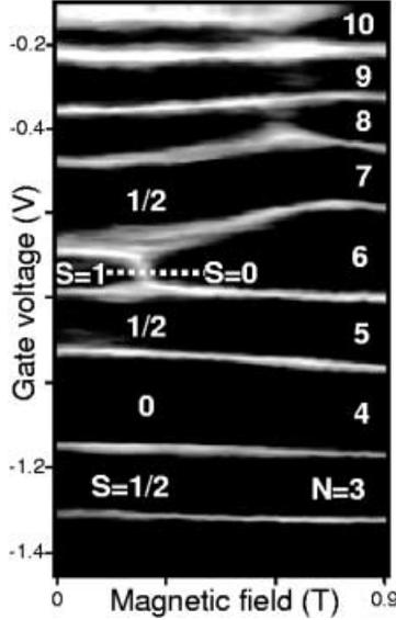
**Fig. 6.** Gray-scale representation of the linear conductance  $G$  versus the gate voltage  $V_g$  and the magnetic field  $B$ . White stripes denote conductance peaks of height  $\sim e^2/h$ . Dark regions of low conductance indicate Coulomb blockade. The  $N = 6$  ground state undergoes a triplet-to-singlet transition at  $B = B^* \approx 0.22$  T, which results in a conductance anomaly inside the corresponding Coulomb gap.
