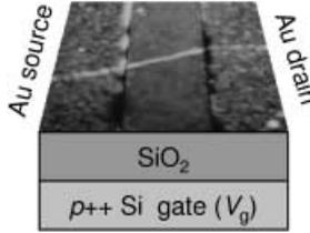
**Fig. 9.** Schematic of a nanotube quantum dot, incorporating an atomic force microscope image of a typical device (not the same one measured here.) Bridging the contacts, whose separation is  $200\text{ nm}$ , is a  $2\text{ nm}$  thick bundle of single-walled nanotubes
