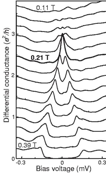
**Fig. 8.**  $dI/dV$  vs  $V$  characteristics taken along the dotted line in Fig. 6 at equally spaced magnetic fields  $B = 0.11, 0.13, \dots, 0.39$  T. Curves are offset by  $0.25 e^2/h$ .
