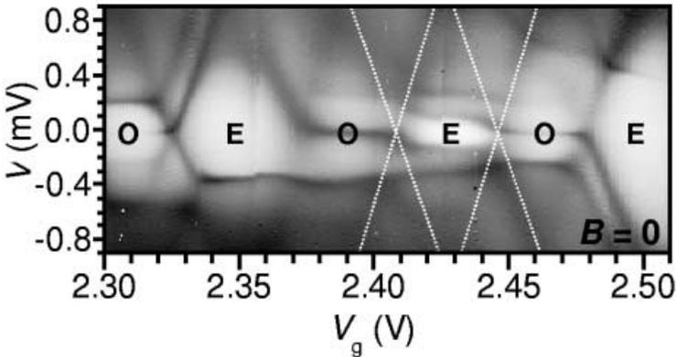
**Fig. 10.** Grayscale plot of differential conductance  $dI/dV$  (darker = more positive) against bias  $V$  and gate voltage  $V_g$  at a series of magnetic fields and base temperature ( $\sim 75\text{ mK}$ ). Labels 'E' and 'O' indicate whether the number of electrons  $N$  in the dot is even or odd (see text).
