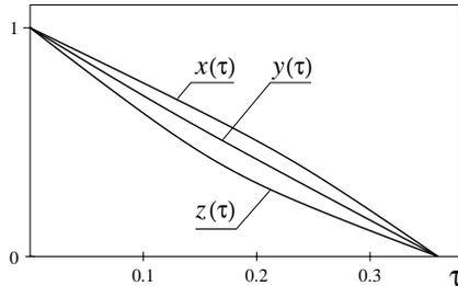
**Fig. 2.** Numerical solution of the scaling equations. The RG equations (16) are rewritten in terms of the new variable  $\tau = \nu J(0) \ln(\delta/D)$  and the new functions  $x(\tau) = J(0)/J(\tau)$ ,  $y(\tau) = I(0)/I(\tau)$ ,  $z(\tau) = V(0)/V(\tau)$  as  $dx/d\tau = -(1 + x^2/y^2)$ ,  $dy/d\tau = -(2y/x + y/z)$ ,  $dz/d\tau = -4z^2/y^2$ . The three functions reach zero simultaneously at  $\tau = \tau_0 = 0.36$ .
