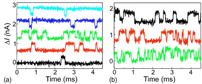
FIG. 2. (Color online) Measured changes in the QPC current,  $\Delta I$ , with the electrochemical potential in the dot and in the reservoir nearly equal.  $\Delta I$  is “high” and “low” for 0 and 1 electrons on the dot respectively ( $V_i = 1$  mV; the steps in  $\Delta I$  are  $\approx 0.3$  nA). Traces are offset for clarity. (a) The dot potential is lowered from top to bottom. (b) The tunnel barrier is lowered from top to bottom.
