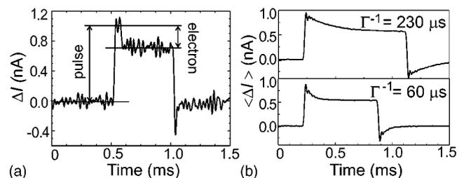
FIG. 3. (a) Measured changes in the QPC current,  $\Delta I$ , when a pulse is applied to gate  $P$ , near the degeneracy point between 0 and 1 electrons on the dot ( $V_i = 1$  mV). (b) Average of 286 traces as in (a). The top and bottom panel are taken with a different setting of gate  $M$ . The damped oscillation following the pulse edges is due to the eighth-order 40 kHz filter.
