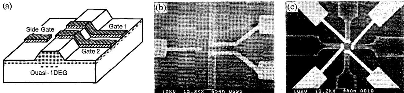
FIG. 1. A schematic illustration (a), and scanning electron micrographs (b) and (c) of two quantum dot samples.
