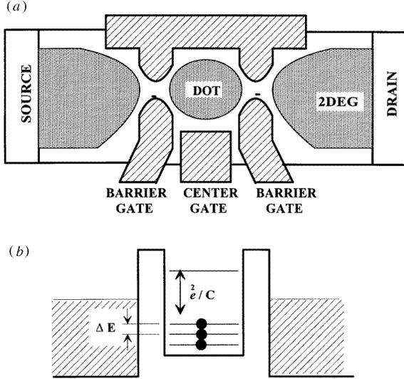
**Figure 1.** (a) Schematic diagram of the device, a gated quantum dot in a GaAs/AlGaAs heterostructure. The dot diameter is approximately  $0.5 \mu\text{m}$ . (b) Schematic energy-level diagram of the dot.
