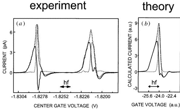
**Figure 2.** (a) Measured  $I-V_g$  with 19 GHz microwaves for  $V_{\text{sd}} \sim 10 \mu\text{V}$ . (b) Calculated  $I-V_g$  for  $V_{\text{S}}^{\text{AC}} = 0.55hf$  and  $V_{\text{D}}^{\text{AC}} = 0.4hf$ ,  $k_{\text{B}}T/hf = 0.1$ ,  $eV_{\text{sd}}/hf = 0.1$ .
