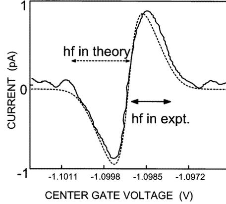
**Figure 3.** Measured (solid) and calculated (dashed) photocurrent at  $V_{\text{sd}} = 0$ . Numerical parameters are  $k_{\text{B}}T = 0.2hf$ ,  $V_{\text{S}}^{\text{AC}} = 0$  and  $V_{\text{D}}^{\text{AC}} = 0.2hf$ .
