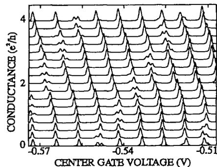
Fig. 2. Coulomb blockade oscillations versus  $V_C$  of dot I from  $B = 4.600 \text{ T}$  (bottom) to  $4.632 \text{ T}$  (top) in increments of 2 mT.
