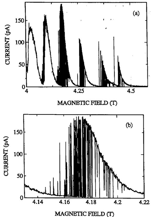
Fig. 4. Conductance through dot II in dependence of magnetic field ((a) and (b)). Peaks occur periodic in one flux quantum added to the dot. Switching is seen at the low-field side of each peak. Note the increase of the switching rate with  $B$ . (b) Expansion of a part of (a).
