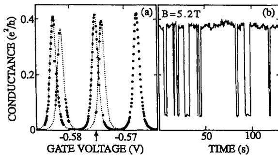
Fig. 3. Conductance of dot I in dependence of (a) the gate voltage  $V_C$  at a fixed field ( $B=5.2$  T) measured with a time constant of 150 ms, and (b) versus time at fixed  $B$  and  $V_C$  (arrow in (a)).
