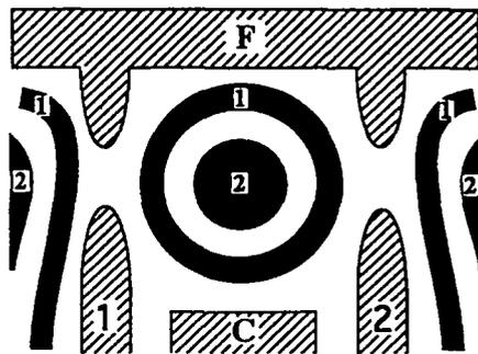
Fig. 1. Schematic diagram of the gate geometry (hatched areas) and the edge states.
