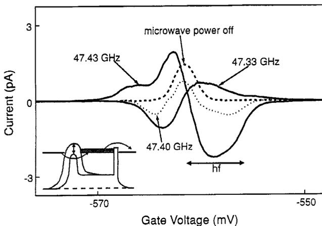
Fig. 3. Measurements of the pumped current at  $B = 1.96 \text{ T}$ ,  $V = 13 \mu\text{V}$  and for frequencies around 47.4 GHz. Dashed line is without microwaves. The dotted line shows the smallest asymmetry, but shows evidence for a pumping mechanism which is not included in our model.
