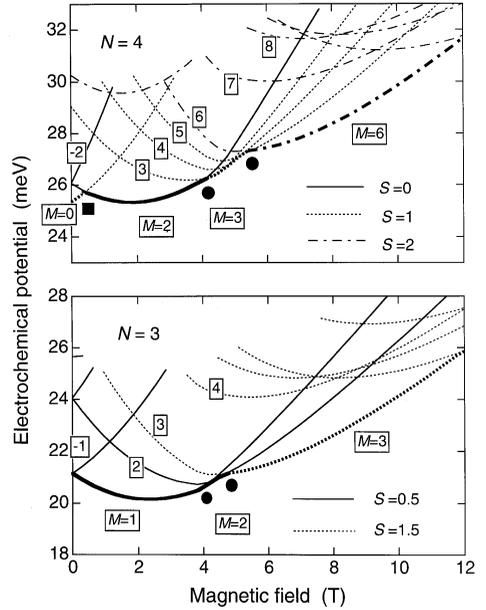
Fig. 6. Exact calculations of ground states (thick lines) and excited states (thin lines) for  $N = 3$  and 4. Many-body states are indexed by the total spin and angular momentum (boxed numbers). For  $N = 3$ , the solid and dotted lines indicate  $S = 0.5$  and  $1.5$ , respectively. For  $N = 4$ , the solid, dotted and dot-dashed lines indicate  $S = 0$ , 1 and 2 respectively. The  $\blacksquare$ ,  $\bullet$  labels are discussed in the text.
