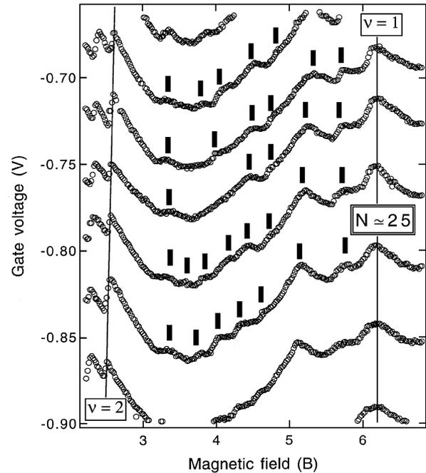
Fig. 3.  $B$ - $N$  phase diagram for device B in the region of  $N \approx 25$  measured in a  $^3\text{He}$  cryostat.  $V_{sd}$  is  $\approx 30 \mu\text{V}$ ,  $V_g$  is varied from about  $-0.9$  V to  $-0.65$  V, and the  $B$ -field is from 2.2 T to 6.8 T. Thick bars mark identifiable features over five consecutive peaks.
