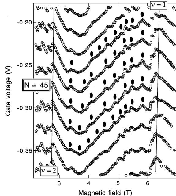
Fig. 4.  $B$ - $N$  phase diagram for device B in the region of  $N \approx 45$  measured in a  $^3\text{He}$  cryostat.  $V_{sd}$  is  $\approx 30 \mu\text{V}$ ,  $V_g$  is varied from about  $-0.35$  V to  $-0.2$  V, and the  $B$ -field is from 2.2 T to 6.95 T. Ovals mark identifiable features over five consecutive peaks.
