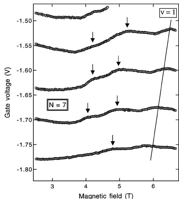
Fig. 2.  $B$ - $N$  phase diagram for device B covering  $N$  from 5 to about 10 measured in a  $^3\text{He}$  cryostat.  $V_{sd}$  is  $\approx 40 \mu\text{V}$ ,  $V_g$  is varied from about  $-1.8 \text{ V}$  to  $-1.5 \text{ V}$ , and the  $B$ -field is from 2.5 T to 6.7 T. Arrows mark weak 'cusps'.
