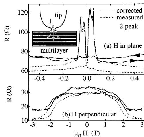
FIG. 1. Magnetoresistance of point contacts to a [Co(2 nm)/Cu(2 nm)]<sub>25</sub> multilayer for the in-plane (a) and perpendicular orientation (b). Dashed lines: as-measured curves. Solid lines: GMR after correction for magnetostriction. Inset: schematic cross section of a contact between tip and multilayer. The contact has a close-to-CPP geometry.
