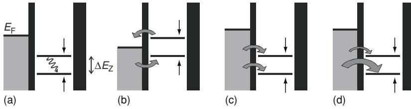
FIGURE 36.2. Schematic energy diagrams depicting initialization procedures in a large parallel or perpendicular magnetic field. (a) Spin relaxation to pure state  $\uparrow$ . (b) The ‘read-out’ configuration can result in  $\uparrow$  faster. (c) Random spin injection gives a statistical mixture of  $\uparrow$  and  $\downarrow$ . (d) In a large perpendicular field providing a strong spin-selectivity, injection results mostly in  $\uparrow$ .
